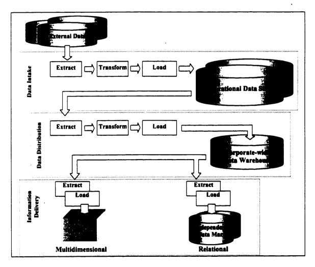
Figure 12: Enterprise-Wide DW with Centralized Data Intake Layer
